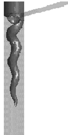
Fig. 6 Computed capturing surface for single phase flow. Q_3=7.8 \times 10^{-3} \text{ m}^3/\text{s} .
