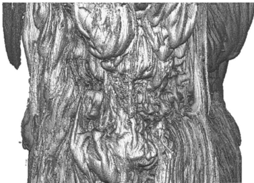
Fig. 2 High-resolution quantitative visualization of a turbulent outer interface derived from space-time \sim 1000^3 measurements of the concentration field in a fully developed liquid-phase jet. The Reynolds number is Re \sim 20,000 and the Schmidt number is Sc \sim 2000 so that the flow conditions are above the mixing transition. The measurements were recorded in the UC Irvine large-scale water tank facility using visible laser-induced fluorescence of dilute disodium fluorescein seeded in water, excited by argon-ion laser illumination. This space-time visualization captures the dynamics of the outer interface with the time axis in the vertical direction. The full transverse spatial extent of the interfaces is captured including the small scales. The interface shown corresponds to a concentration threshold of c/c_1 = 1 , cf. Figs. 11 and 12.
