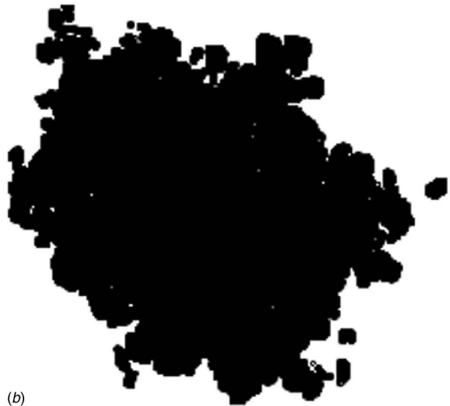
Fig. 4 Examples of the regions of mixed fluid (black) in the single-stream shear layer (top) and in the jet (bottom). The boundaries of the mixed-fluid regions correspond to the outer interfaces separating mixed fluid shown in black from the pure fluid(s) shown in white.
