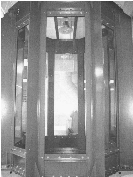
Fig. 7 Photograph of the water tank facility at UC Irvine. The tank is octagonally shaped with an internal height of 2.74 m (6 ft) and a diameter of 1.83 m (9 ft). The capacity of the tank is 8 tons or 2000 gallons of water. The tank has extensive optical access by way of eight vertical 0.61 m by 2.13 m (2 ft by 7 ft) windows and one horizontal 0.61 m (2 ft) diameter window at the base. The large size of the tank facilitates large-scale high-resolution imaging of the concentration field while at the same time enabling flow conditions above the mixing transition.
